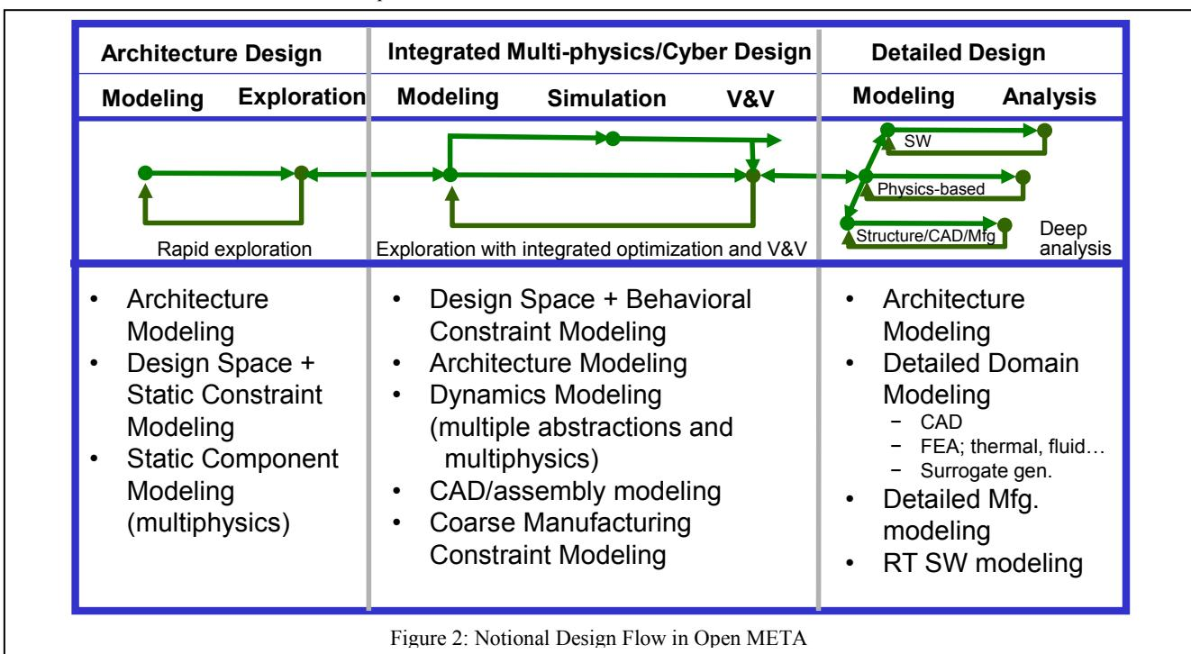
Figure 2: Notional Design Flow in Open META
