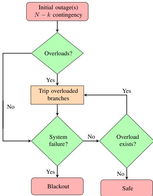
Fig. 3: Cascade Simulation Model
