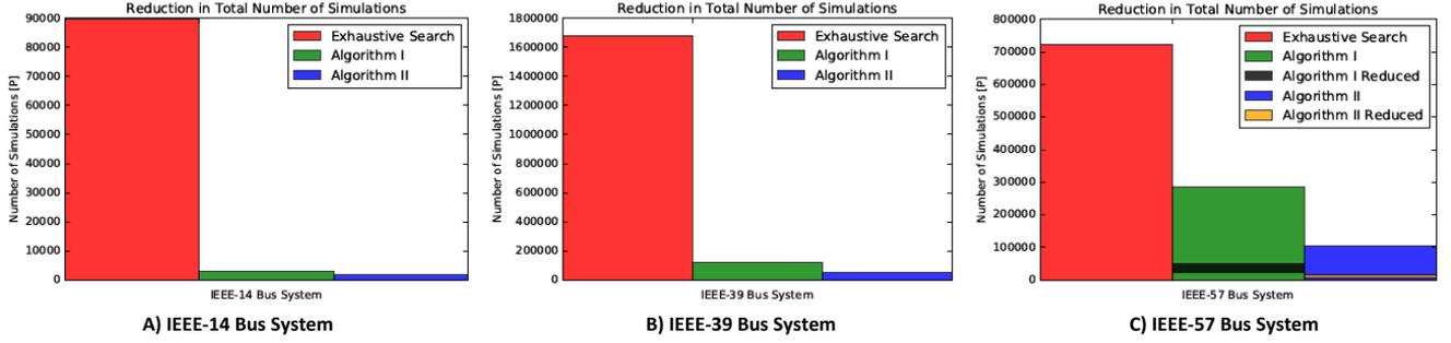
Fig. 5: Total Number of Simulations Run using Exhaustive Search, Algorithm I and Algorithm II to Identify Critical  $N - k$  Contingencies
