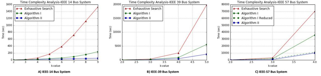
Fig. 4: Execution Time Analysis-Time taken by Exhaustive search, Algorithm I and Algorithm II to Identify Critical  $N - k$  Contingencies
