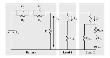
Fig. 5. Schematic diagram for the battery system.
