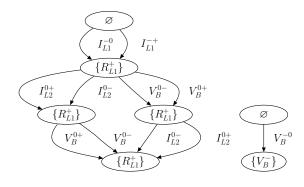
Fig. 6. Fault models for the battery system.
