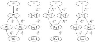
Fig. 3. Diagnosers for the individual faults of the circuit. The diagnosers for decreases in the parameter values are the same except for a reversal in the signs.
