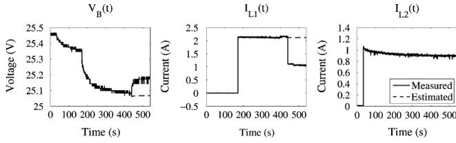
Fig. 11.  $R_{L1}^+$  fault, where  $R_{L1}$  increases by 100%.
