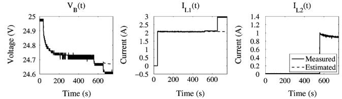
Fig. 9.  $R_{L1}^-$  fault, where  $R_{L1}$  decreases by 33%.
