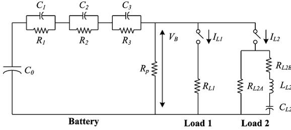
Fig. 7. Electrical circuit equivalent for the battery system.
