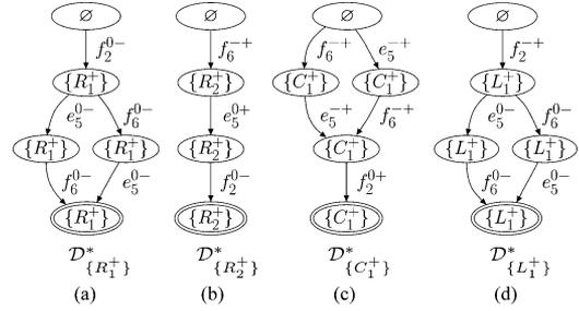
Fig. 5. Diagnosers for the individual faults of the circuit. The diagnosers for decreases in the parameter values are the same except for a reversal in the signs.
