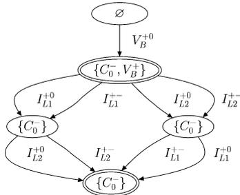
Fig. 14. Partial diagnoser for isolating the  $V_B^+$  fault.
