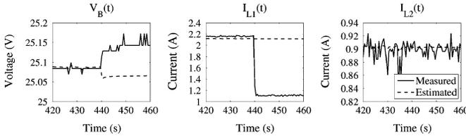
Fig. 12. Detailed plot of  $R_{L1}^+$  fault.
