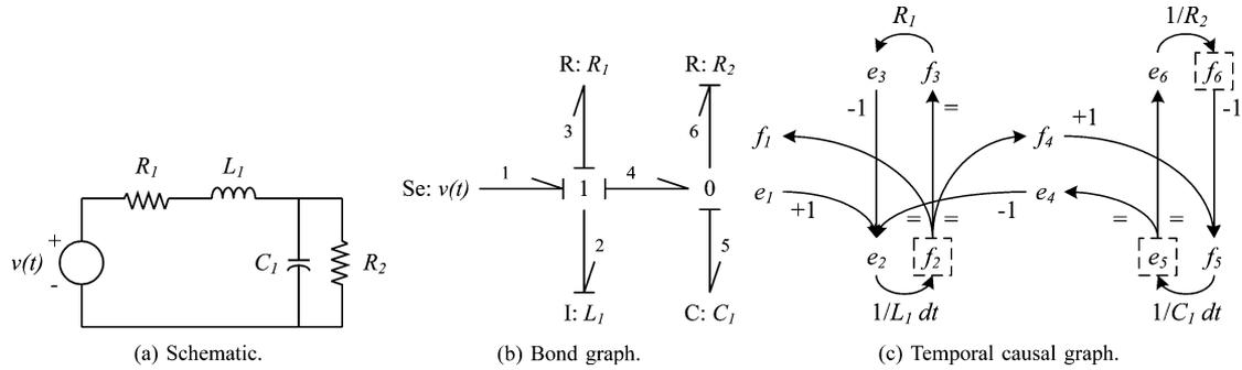
Fig. 1. Circuit example. (a) Schematic. (b) Bond graph. (c) Temporal causal graph.
