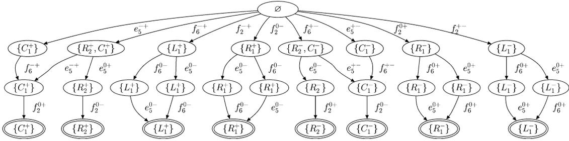
Fig. 6. Event-based diagnoser for the circuit.
