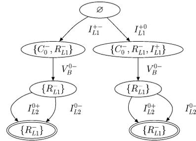
Fig. 10. Partial diagnoser for isolating the  $R_{L1}^-$  fault.
