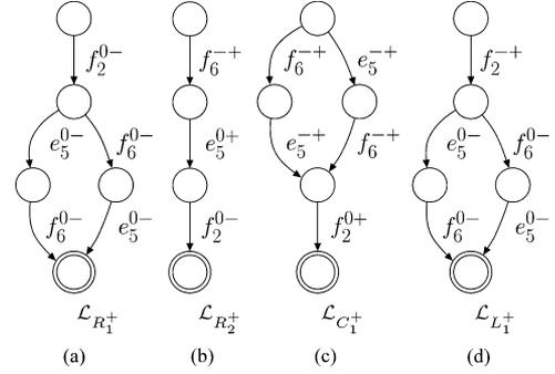
Fig. 4. Fault models for the faults of the circuit. The fault models for decreases in the parameter values are the same except for a reversal in the signs.
