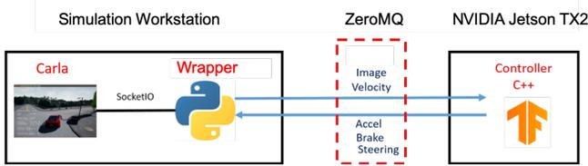
Fig. 4: Testbed Setup
