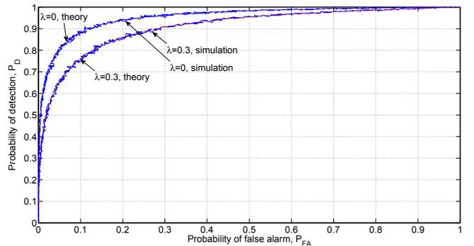
Fig. 3. ROC curve-Z-test with intermittent observations-Monte Carlo simulations and analytical results.
