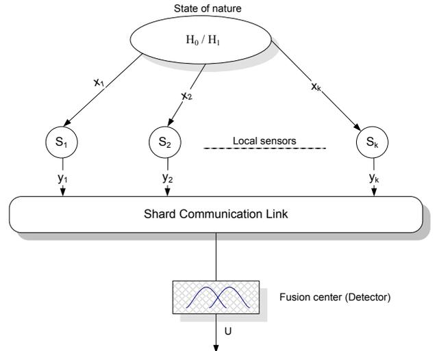
Fig. 1. Detection with intermittent observations. The shared communication link may represent a wired communication cable, or a wireless channel. The detector is to decide on one of two states of nature.
