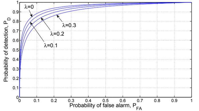
Fig. 2. ROC curve-Z-test with intermittent observations. The performance degrades with the increasing percentage of channel drop rate,  $\lambda$ .
