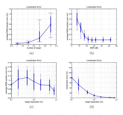
Figure 3: Localization error with (a) Source density, (b) Source SNR, and (c) Source separation. (d) Localization error as a percentage of source separation.
