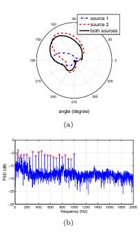
Figure 1: (a) Acoustic Beamforms; The beamforms for single sources clearly show peaks at the source location but the beamform when both sources are present does not show two peaks. (b) Power spectral density (PSD); The highest PSD values are shown as empty circles. The PSD is compactly represented as pairs of the highest PSD values and corresponding frequencies.
