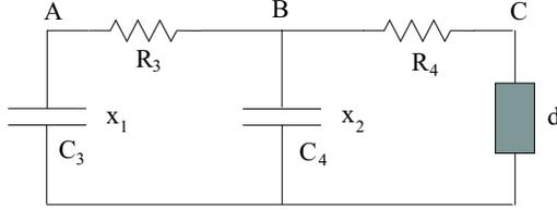
Figure 2: Electric circuit describing the case when the furnace is off.
