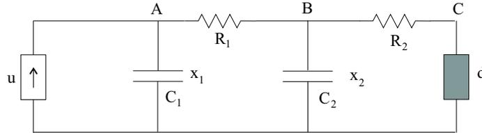
Figure 1: Electric circuit describing the case when the furnace is on.
